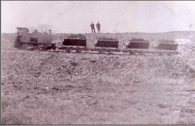
Very few new photos have come to light but when they do they can reveal a lot. This one was thought to show a train in one of the quarries but it is actually on the tip north of Dimple Lane by the Hat Factory, the triangle of track in the foreground was just north of the Warner Quarry branch. This shows that the later locomotives were capable of running up the steep gradients on the tip sidings and that side tip wagons were in use for this purpose. (Photo copyright Alan C.Baker)
